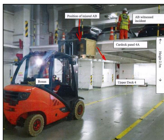
Figure 3: Simulated photo showing deck 4, hoistable car deck 4A, and position of crew members prior to the accident.
