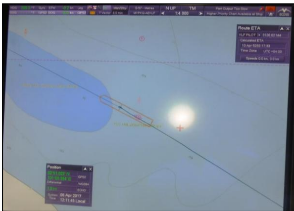
Figure 1: Screenshot from the ECDIS showing vessel heading in shallow water
