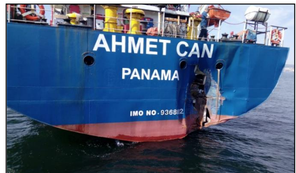
Figure 8: Photo showing damage sustained by Ahmet Can
