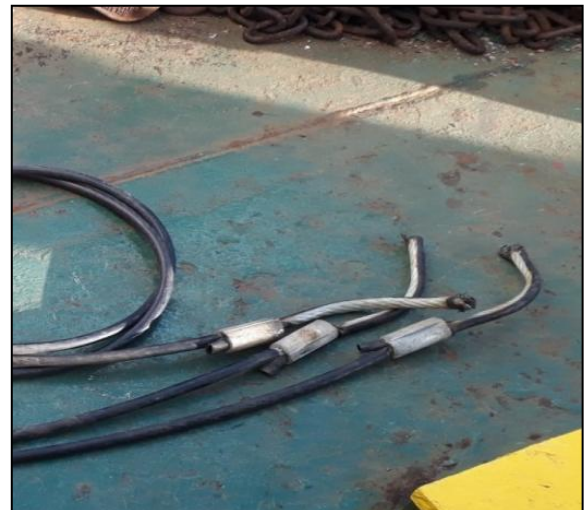
Figure 6: Showing three of four damaged hoisting slings that were connected to the floating beam unit
