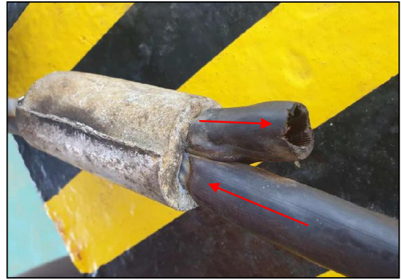
Figure 7: Sheathing passed through the ferrule in both directions
