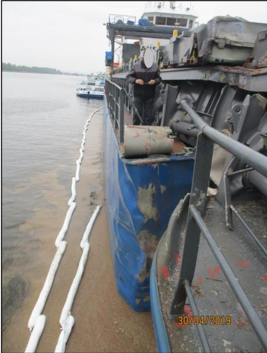
**Figure 8: Linseed cargo spilled from the cargo hold**
