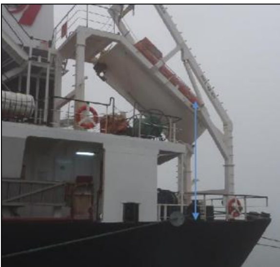
Figure 3: The drop from the davits to the poop deck was about 4.0 m
