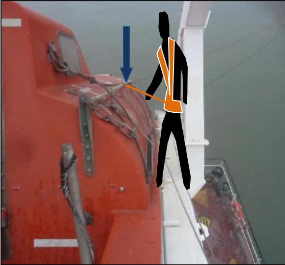
Figure 2: Blue arrow shows where the safety harness was attached to the lifeboat's railing
