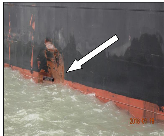
Figure 4: Fractured section of the hull plugged by the crew
