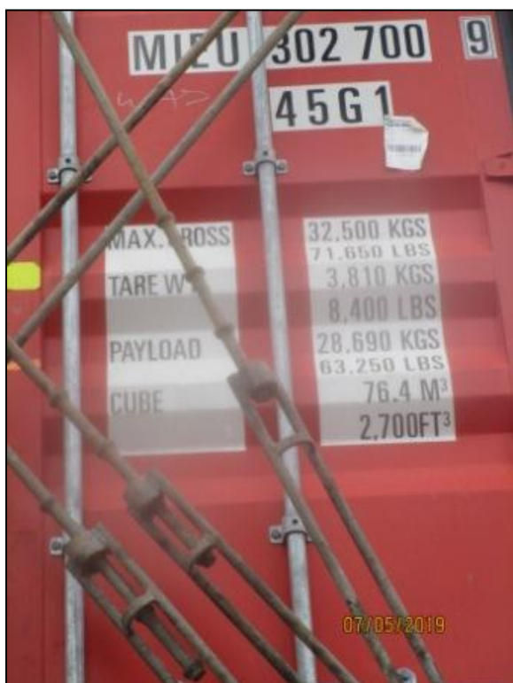
Figure 6: A lashing bar connected to a turnbuckle
