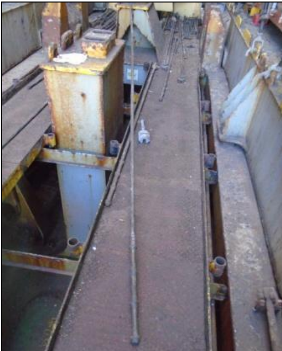
Figure 2: Long lashing bar used for securing
