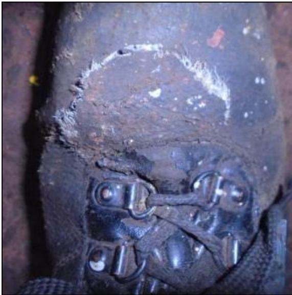
Figure 9: The safety shoe of the injured seafarer, after the accident
