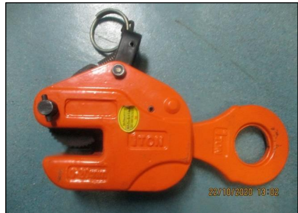
Figure 9: A lifting clamp on board Miss Benedetta
