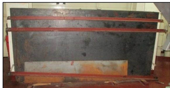
Figure 5: Securing arrangement of the stack
