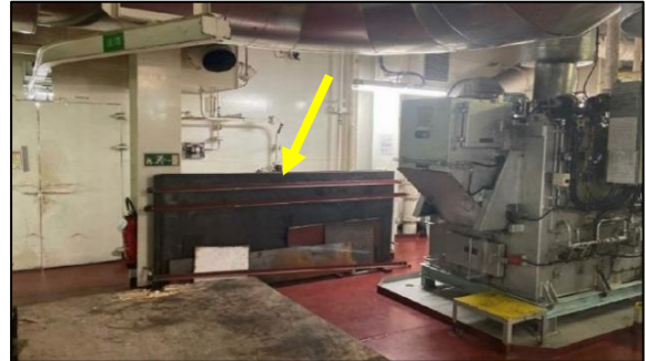
Figure 3: Location of the secured stack of spare steel plates in the engine-room
