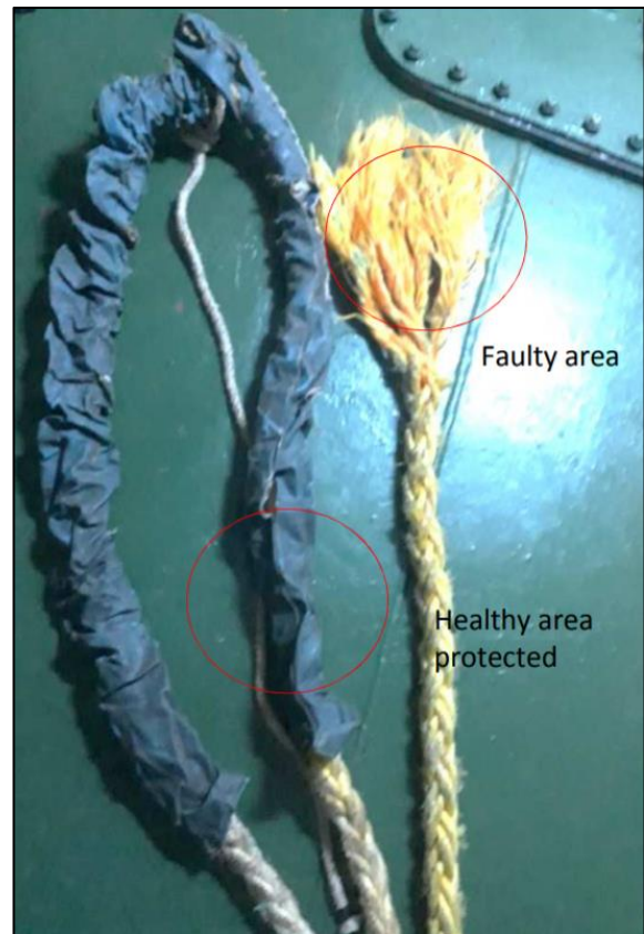
Figure 4: Area of the mooring rope under optical and SEM/EDX analysis
